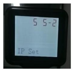
**8.2.5** Enter the IP of your company's LAN (the last three digits should avoid duplication with other devices. For example, my IP is 192.168.100.44, and the IP I set on the scale is 192.168.100.123)
