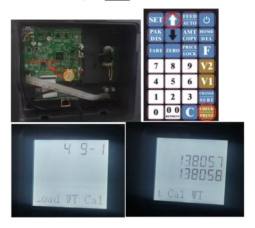
9.7 Put 5kg calibrated weight on the plate, then press check to confirm the calibration.
