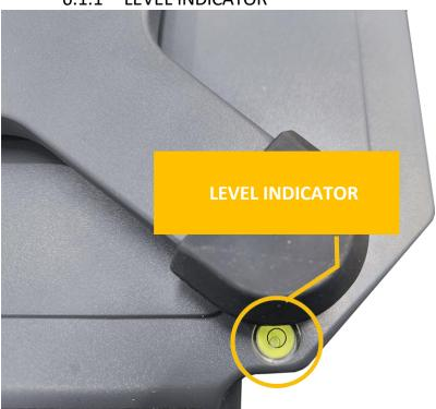
The level indicator is located below the scale pan. When the bubble leaves the center and its edge contacts the black inner ring, it indicates that the maximum allowable inclination is exceeded and it is prohibited to use. Please adjust the scale foot so that the bubble of the level indicator is in the middle of the black inner ring before continuing to use.
