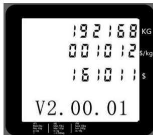
Figure 2 start self-test step 2: IP address and version number.
